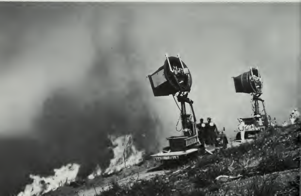
Large fans have been used experimentally to control fires in heavy brush.
